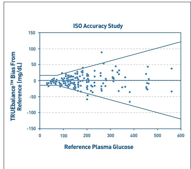
TRUEbalance™ System meets the ISO criteria for accuracy with 96.5% of results within the limits
