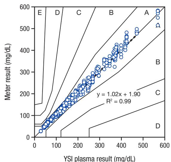
A, Bias plot of all TRUE METRIX® GO results versus YSI reference instrument results analyzed per the ISO 15197:2013 accuracy standard.
