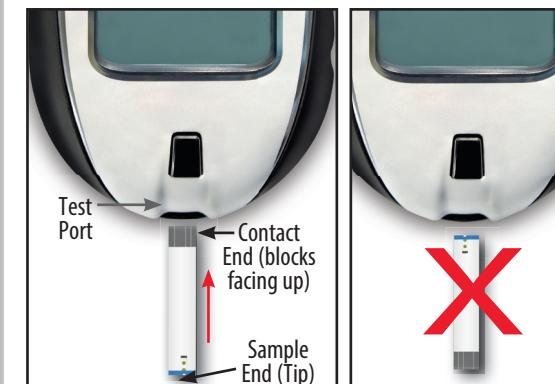
With meter off, insert Test Strip into Test Port with Contact End (blocks) facing up. The Meter turns on.
