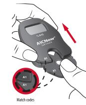
If analyzer and cartridge codes do not match cal Customer Service at 1-877-870-5610.
