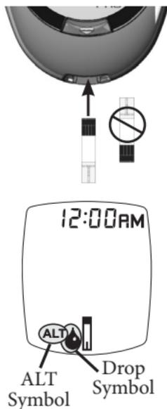
**Note:** If test strip has been out of the vial too long before testing, an error message appears upon insertion of the test strip into the meter. Release and discard old test strip. Use new test strip for testing.
