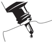
9. With test strip still in meter, touch edge of Sample Tip to top of drop of control solution. Allow drop to be drawn into test strip. Remove test strip from drop when meter beeps.
