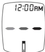
10. After the test is finished, result is displayed. The Strip Release Button flashes. Record result as required by your facility.
