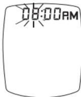
3. The minutes flash. Press “▶” or “◀” Button to set the minutes. Press “•” Button to set. Meter goes to the next Test Reminder.
