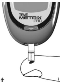
8. With test strip still in meter, touch Tip of test strip to top of blood drop and allow blood to be drawn into test strip. Remove Sample Tip from blood drop immediately after the meter beeps and dashes appear across the meter Display.
