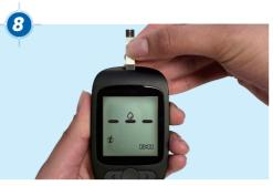
With meter off, insert test strip contact end (blocks facing up) into Test Port. Meter turns on. Keep test strip in meter until testing is finished.
