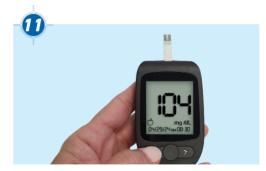
After a 5-second count down, meter displays the test result.
